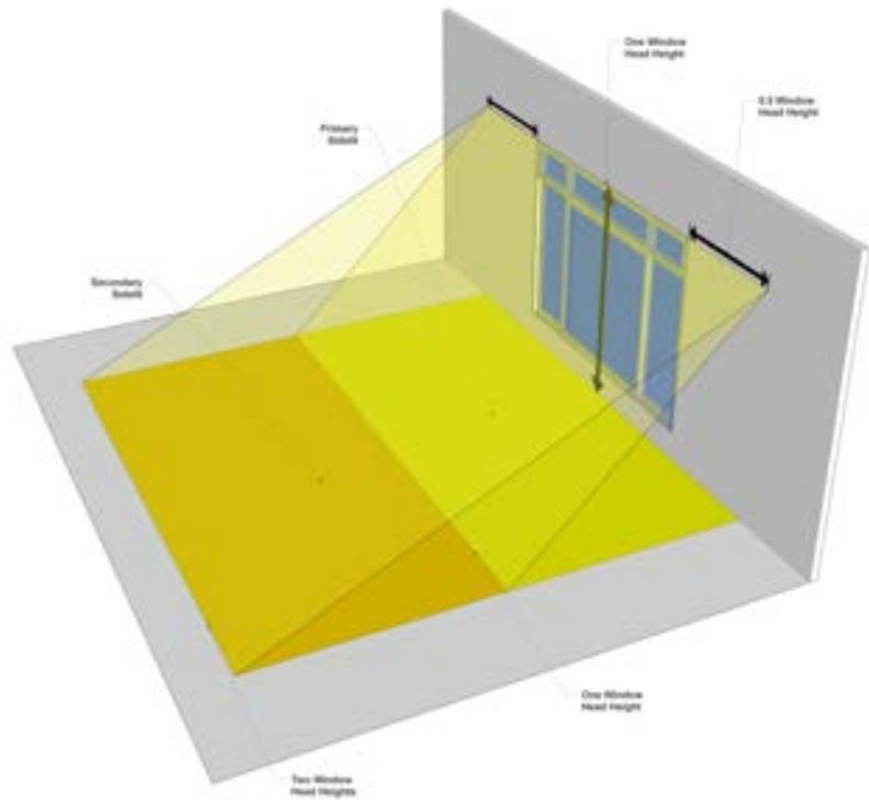
Sidelit Daylit Zones – The sidelit daylit zones extend one and two window head heights into the room, and their width is the width of the window plus  $\frac{1}{2}$  the window head height in each direction.
