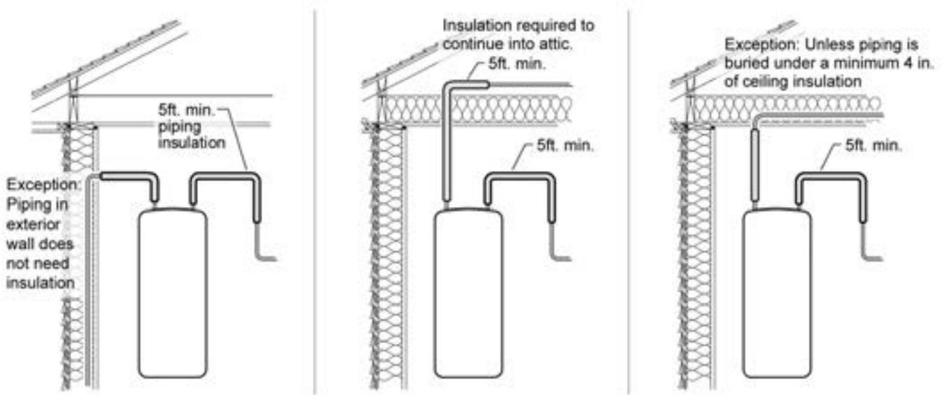
Pipe Insulation – Pipes embedded in insulation in walls, and piping in ceilings where buried under at least 4 inches of insulation, are not required to be insulated.
