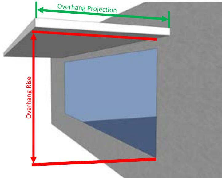
Overhangs – Overhangs can limit the amount of daylight that enters a space. For South, East, and West-facing fenestration, if the overhang projection-to-rise ratio is 1.5 or greater, the area adjacent to that fenestration is exempt from the daylighting control requirements. For north-facing fenestration, these areas are exempt if the overhang projection-to-rise ratio is 1.0 or greater. This is detailed in Exception 2 to Section 130.1(d) of the Energy Code. Source: California Energy Commission
