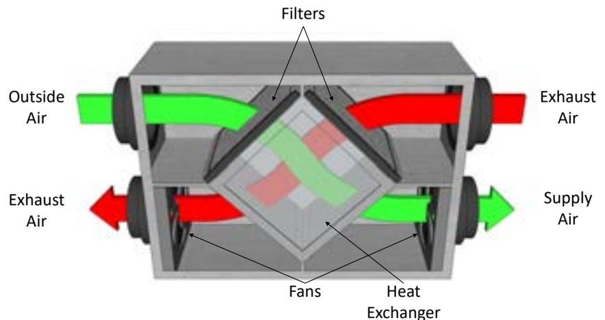
Energy Recovery Ventilator – The supply air (green arrow) must pass through a MERV 13 filter.
