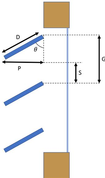
Horizontal Slats – To qualify for a lighting power adjustment factor, horizontal slats must meet the requirements of Section 140.6(d)2. Source: California Energy Commission
