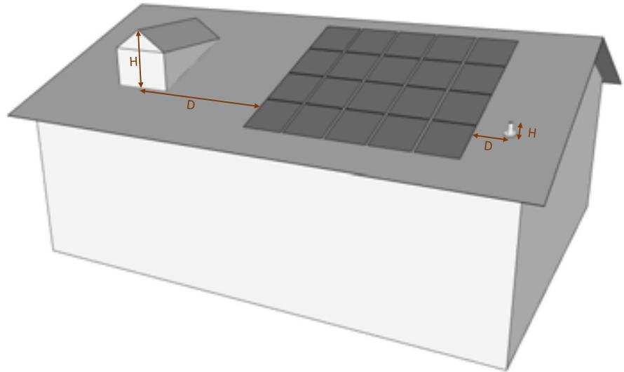
Solar Ready Shading Limitations – In order to comply with the shading limits, in this illustration, the distance (D) between the peak of the potential shading object and the solar panels must be twice the height (H) of that peak.
