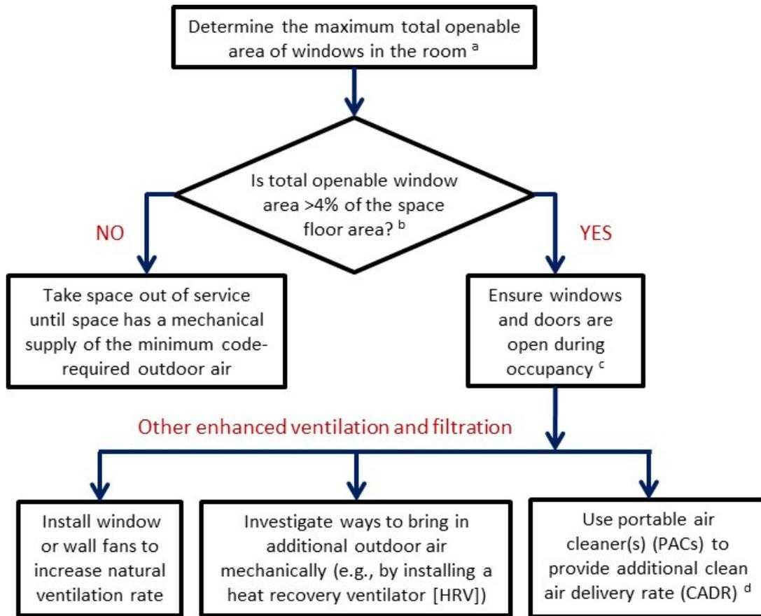
Figure 1. Flow chart for checking spaces without mechanical ventilation.
