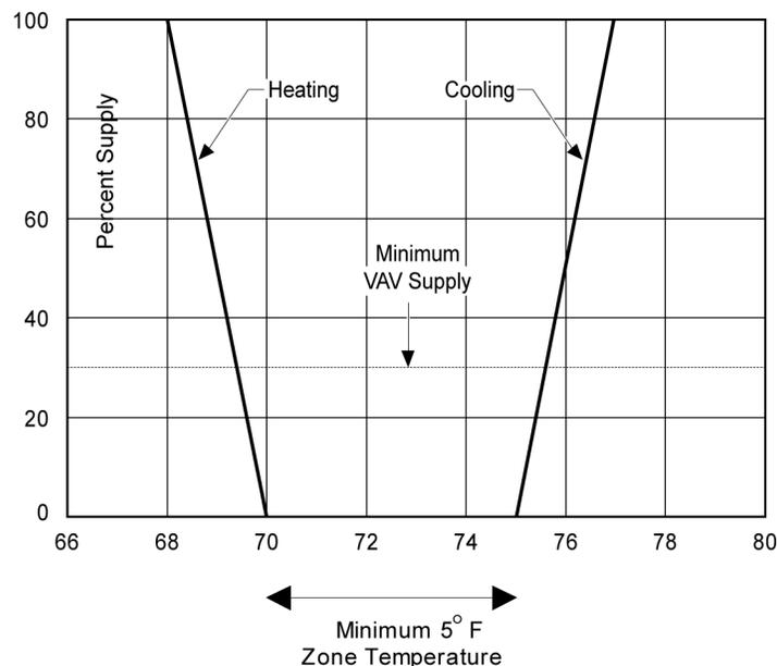
Supplemental perimeter heating or cooling systems are sometimes used to augment a space-conditioning system serving both interior and perimeter zones. This is allowed provided controls are incorporated to prevent the two systems from conflicting with each other. If that were the case, then the Energy Standards require that:
