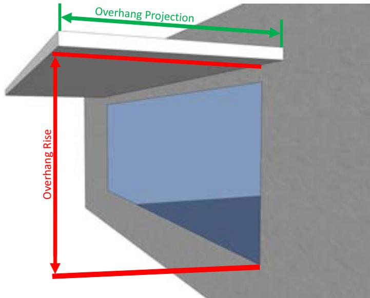
Overhang Rise – The “overhang rise” is depicted by the red arrow. It is the vertical distance between the projected edge of an overhang and the window sill below.
