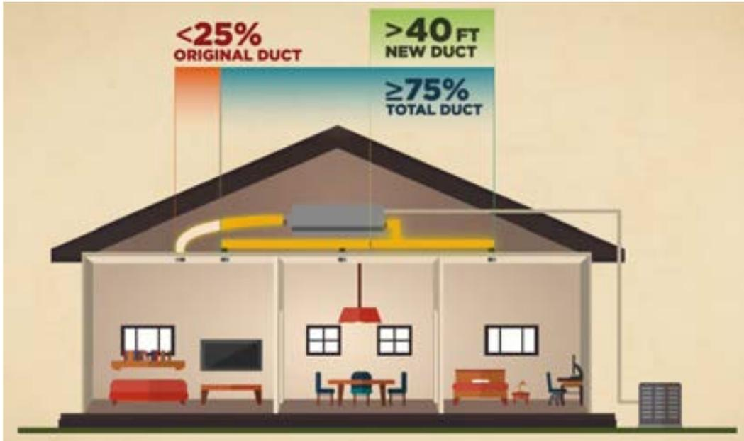
Duct Alteration Triggers – If more than 40 linear feet of new or replacement space-conditioning ducts are installed, then duct leakage testing and prescriptive insulation requirements are required. When 75 percent or more of the duct system is replaced, this is considered a complete replacement of the duct system, which has more stringent requirements as described in Section 150.2(b)1Diia of the Energy Code.
