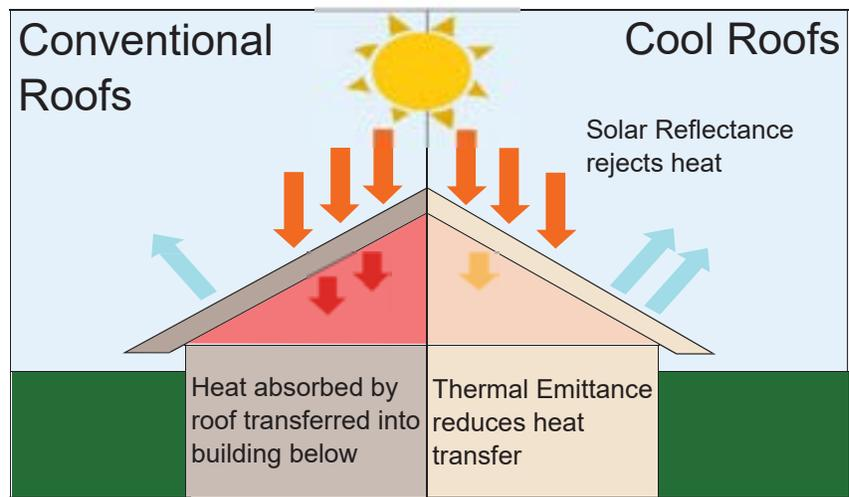
Solar Reflectance and Thermal Emittance: Solar reflectance rejects heat, while thermal emittance reduces heat transfer.
