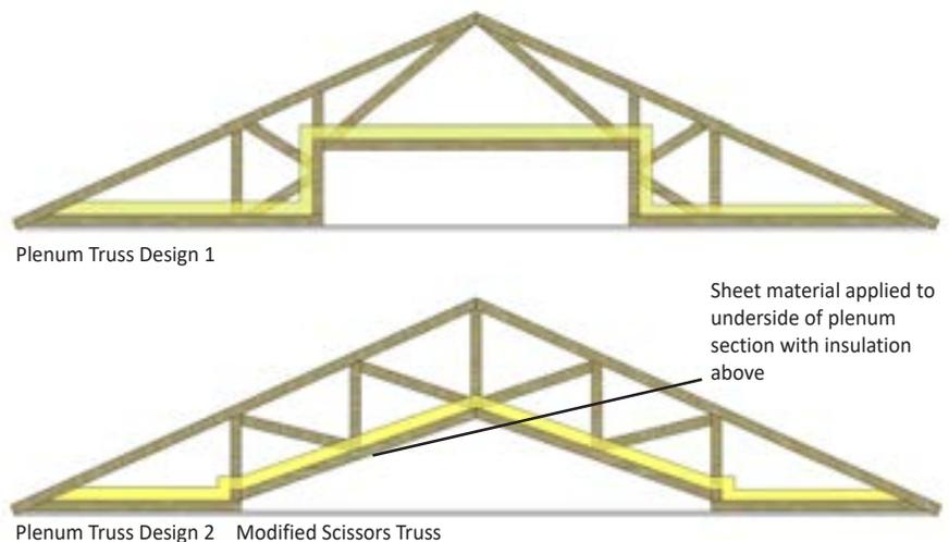
Indirectly Conditioned Attic Spaces – The spaces below the yellow insulation but above the ceiling line are considered indirectly conditioned spaces.
