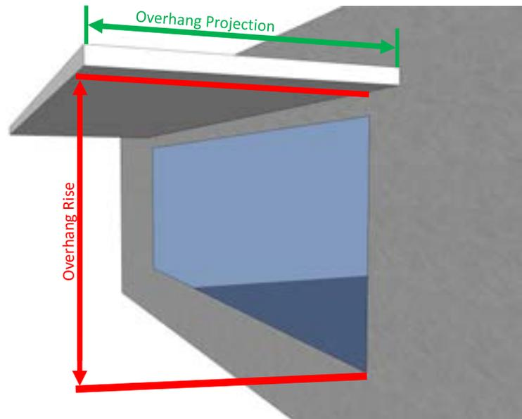
Overhangs – Overhangs can limit the amount of daylight that enters a space. For South, East, and West-facing fenestration, if the overhang projection-to-rise ratio is 1.5 or greater, the area adjacent to that fenestration is exempt from the daylighting control requirements. For north-facing fenestration, these areas are exempt if the overhang projection-to-rise ratio is 1.0 or greater. This is detailed in Exception 3 to Section 140.6(d) of the Energy Code.
