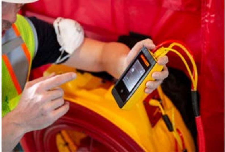
HERS Verified Blower Door Test – Envelope leakage, when modeled, must be verified by a third party HERS rater. Source: California Energy Commission
