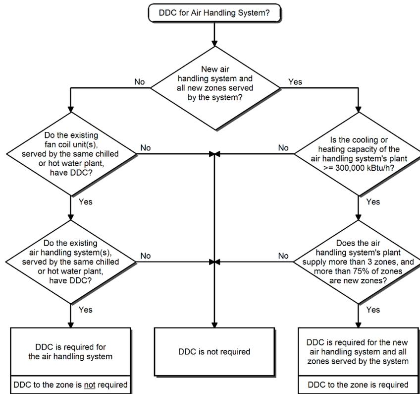
Figure 4-18: Zone Terminal Unit Flowchart
