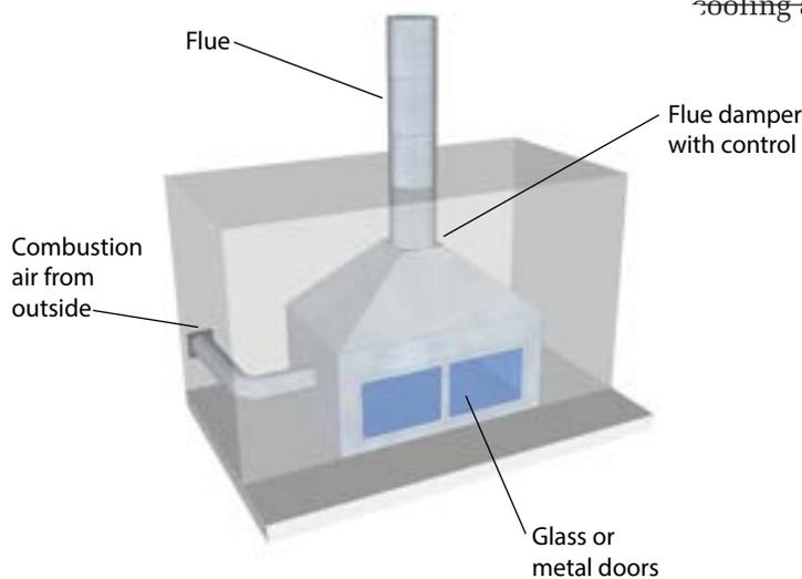
Gas Fireplace – The CALGreen Code requires that gas fireplaces be direct-vent sealed combustion type. The Energy Code also requires that these fireplaces have closeable metal or glass doors.
