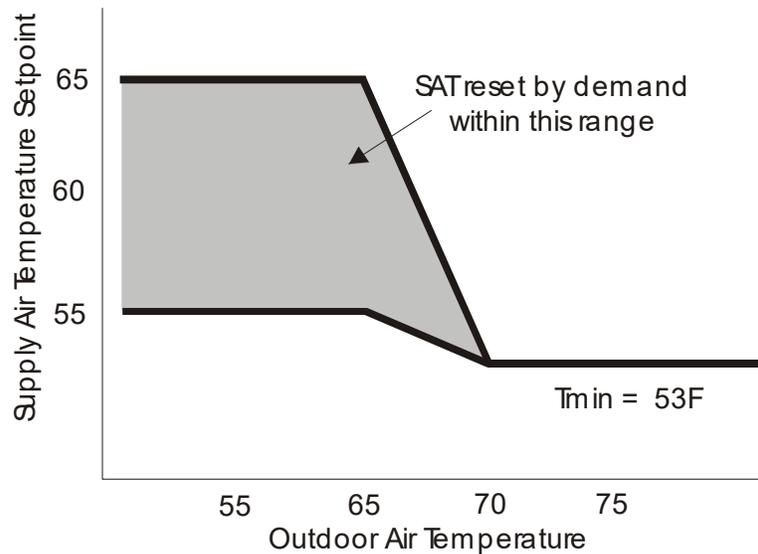
*Recommended Supply Air Temperature Reset Method*
