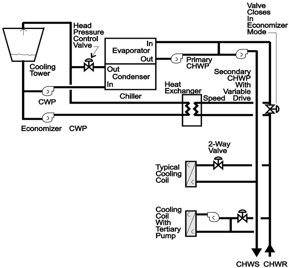
Figure 4-37: Air-Precooling Water Economizer
