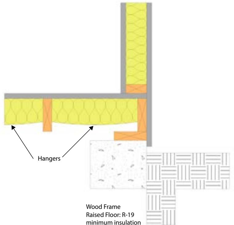
Raised Floor Insulation – R-19 is the mandatory minimum insulation requirement for wood-framed raised floors. Alternatively, a maximum assembly *U*-factor of 0.037 satisfies the mandatory insulation requirement of Section 150.0(d). In this illustration, hangers are used to hold insulation in place.
