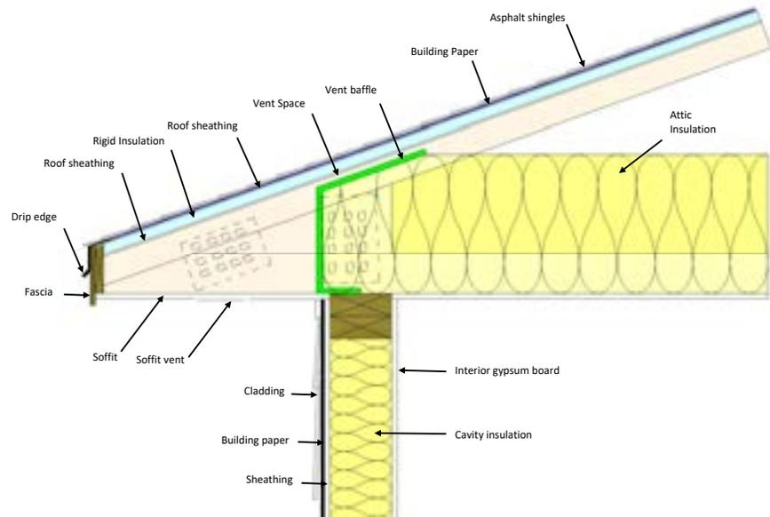
High-Performance Attic with Insulation Above Rafters – This prescriptive option for compliance with the high-performance attic requirements has been removed from the 2019 Energy Code. When complying via the performance approach, installing insulation above the roof rafters is still acceptable, and can be modeled for compliance.
