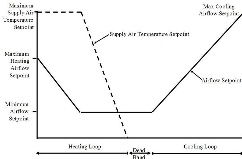
For systems without DDC to the zone (such as electric or pneumatic thermostats), the airflow that is reheated is limited to a maximum of the larger either 30 percent of the peak primary airflow or the minimum airflow required to ventilate the space.
