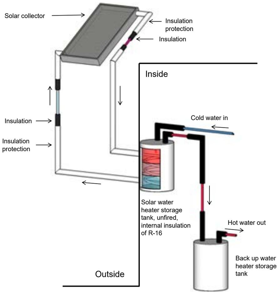
Solar Water Heating System – The solar water heating collector loop (illustrated on the left, or “outside” area) must be insulated under the 2019 Energy Code. This insulation must also be protected from damage due to sunlight, moisture, equipment maintenance, and wind, where applicable, per Sections 150.0(j)3 and 120.3(b) of the Energy Code.
