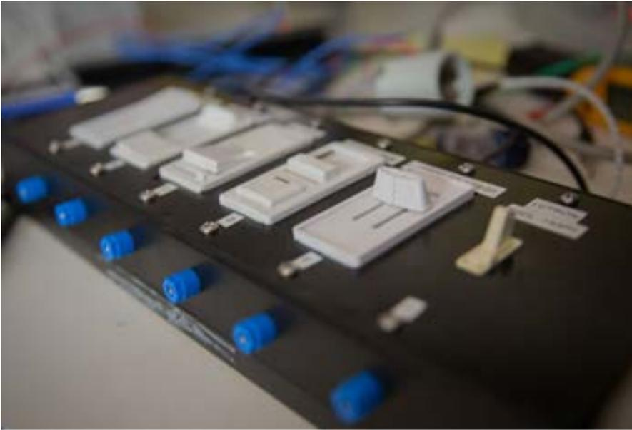
Manual Area Control Options – Depending on the space size, connected lighting load, and space type, Section 130.1(b) of the Energy Code details when the area control for a space must be a dimmer.
