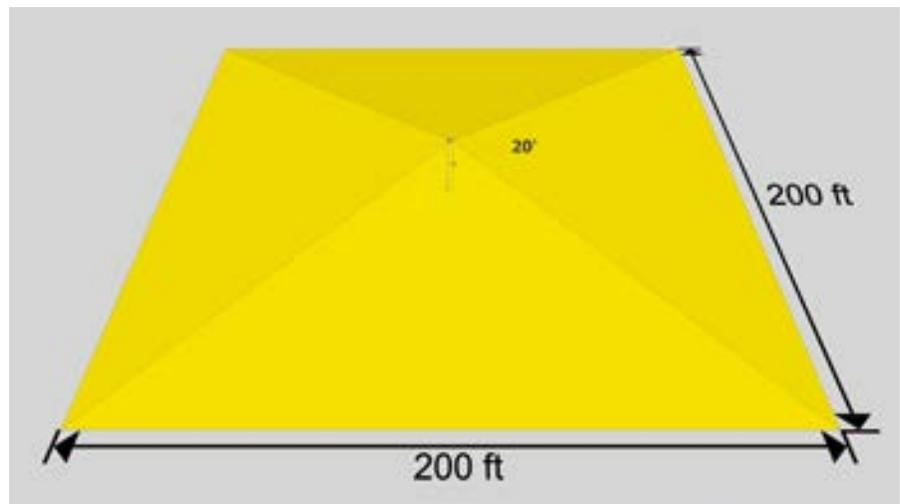
Illuminated Hardscape Area – This is defined as the improved area within a square pattern around each luminaire with each side ten times the luminaire mounting height with the luminaire in the middle of the pattern.
