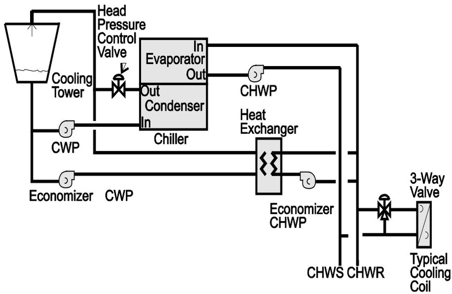
Figure 4-36: Water-Precooling Water Economizer with Two-Way Valves
