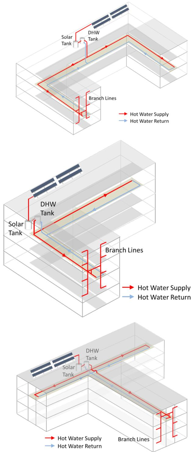
Location of water heating equipment in the building should be carefully considered to properly implement the dual-loop design. The goal is to keep overall pipe length as short as possible, as an example, for buildings that do not have complicated floor plans; the designer should consider locating the water heating equipment at the center of the building footprint rather than at one end of the building which helps to minimize the pipe length needed. If a
