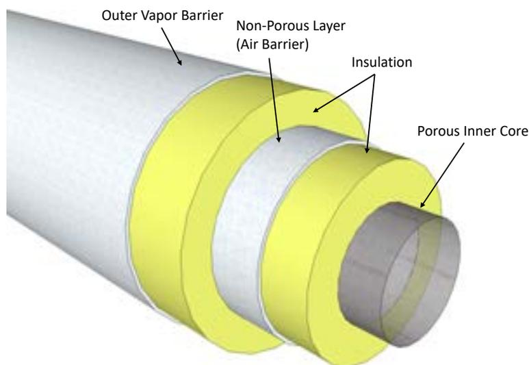
Porous Inner Core Flex Duct – Flexible ducts having a non-porous layer between the porous inner core and the outer vapor barrier satisfy the intent of Section 150.0(m)10 and can be used for compliance with the Energy Code.
