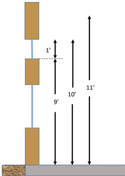
Clerestory – To qualify for a lighting power adjustment factor, clerestory fenestration must meet the requirements of Section 140.6(d)1.
