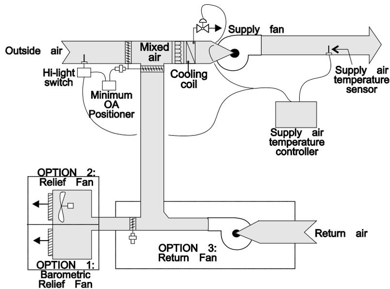
**Figure 4-22: Typical Air-Side Economizer Control Sequencing**
