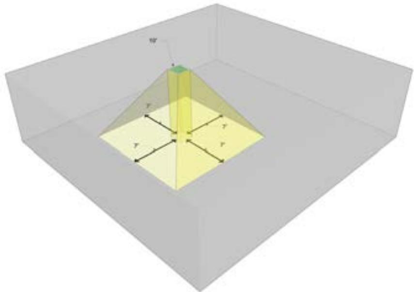
Skylit Daylit Zones – Skylit daylit zones are determined by projecting the skylight to the floor, and then projecting that pattern in each direction a length of 0.7 times the ceiling height. In this example, the ceiling height is 10 feet, and the pattern is extended 7 feet in all directions.
