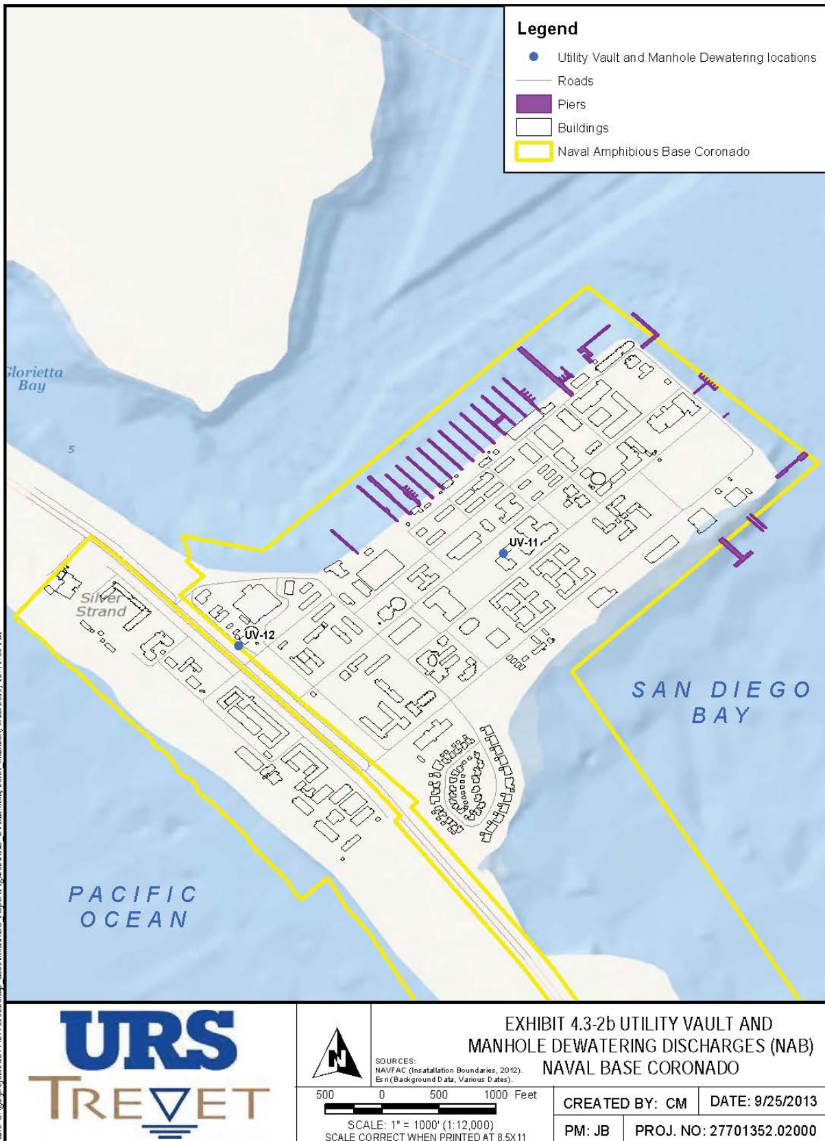
Figure B-7. NBC Utility Vault and Manhole Dewatering Discharge Locations at NAB
