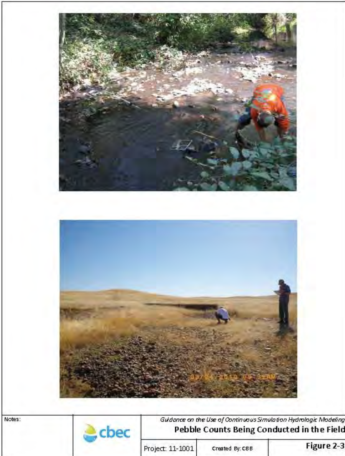
Figure 2-3. Pebble Counts Being Conducted in the Field
