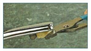
• One or more parts are contained within the aerator. Note the order and orientation of the parts as you remove them;
