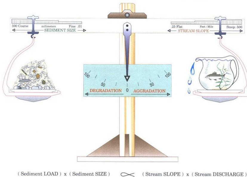
**Figure 5 - Schematic of the Lane Relationship**
