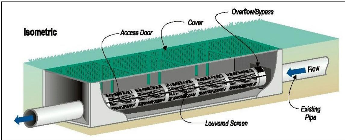
**Figure 3-7 Linear Radial GSRD**
