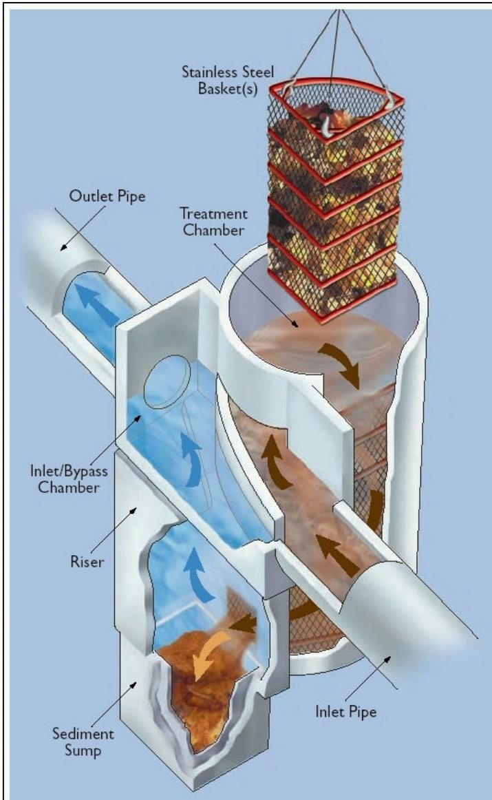
**Figure 3-3 Cleansall™ Gross Pollutant Trap Schematic**
