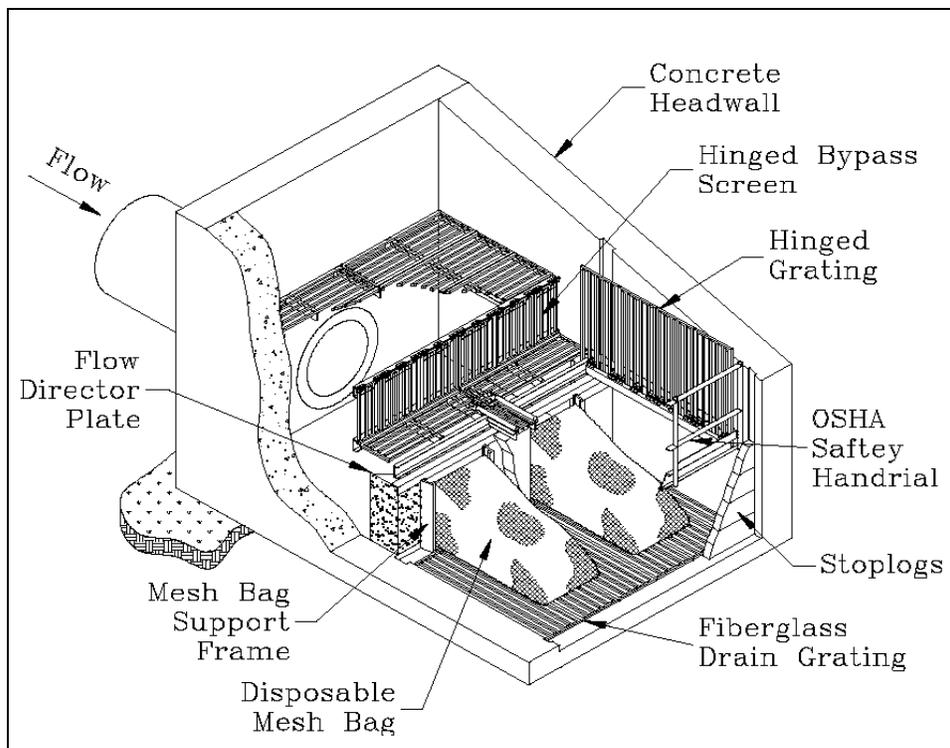
**Figure 3-1 Fresh Creek Netting Trash Trap® End-of-Pipe Schematic**
