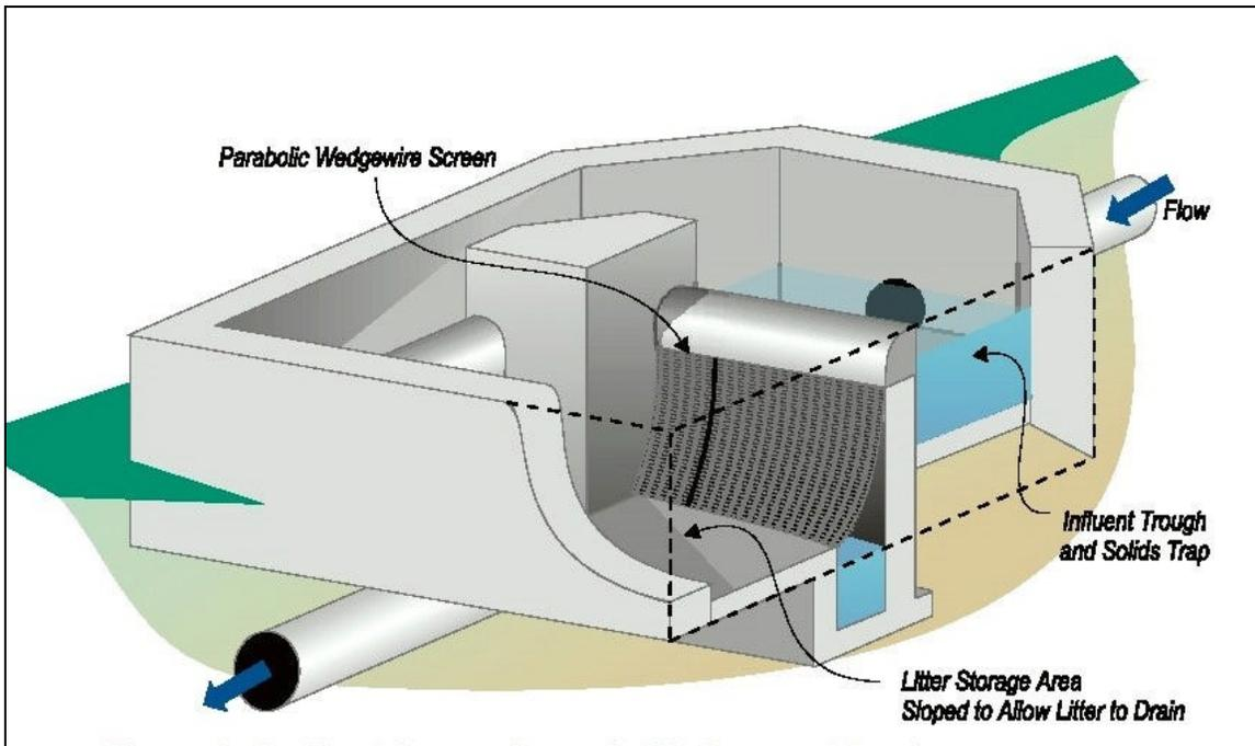
**Figure 3-8 Inclined Screen GSRD**
