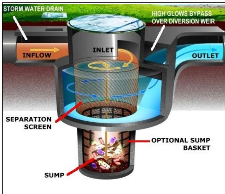
**Figure 3-9 CDS™ Unit Schematic**
